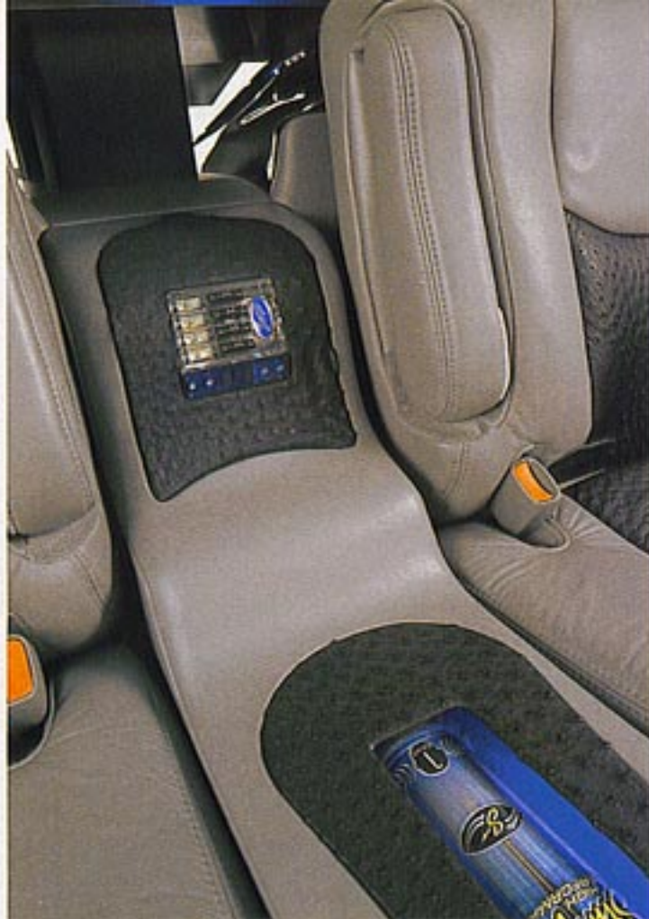
Fuse-lage: At the far end of the added-on center console is a Stinger fused power-distribution block with an LED readout (above).
