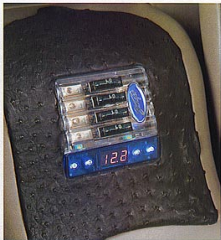
Fuse-lage: At the far end of the added-on center console is a Stinger fused power-distribution block with an LED readout (above).
