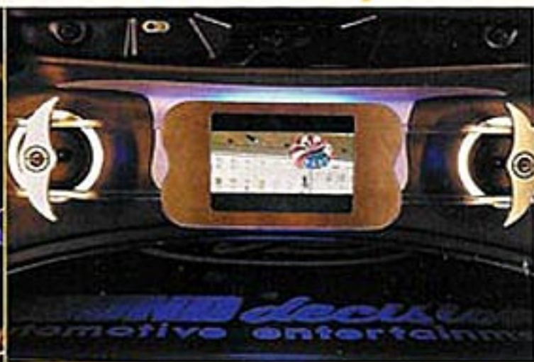
The aluminum Sean Young used to laminate the bars connecting the monitor and tweeters actually carry the signal for the tweeters.
