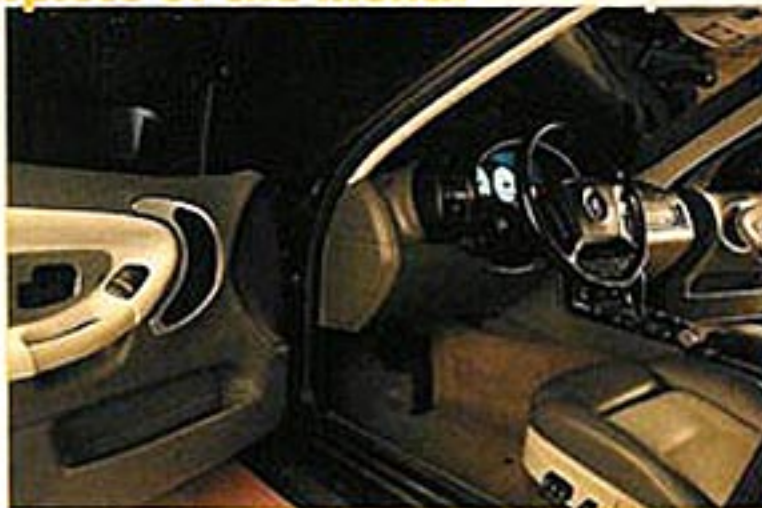
Two-tone Ultra leather radiates throughout the vehicle, as seen with the seats and door panels. Installer Sean Young also added Plexiglas inserts for the door, which were laminated in brushed aluminum. In addition, Young backlit the inserts with neon rope. The installer also fabricated grilles for the four-inch midrange woofer and tweeter mounted inside the door.
